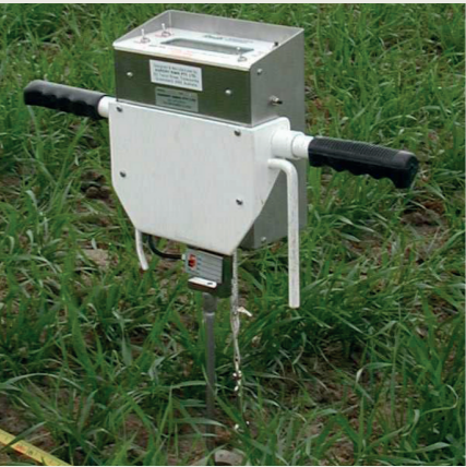
Figure 9. A cone penetrometer that has been pushed into the soil to collect soil strength readings under a wheat crop.
