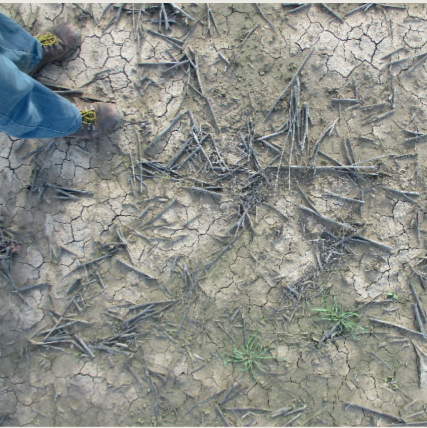
Figure 12. Typical surface flake formation seen in a sodic clay following rainfall
