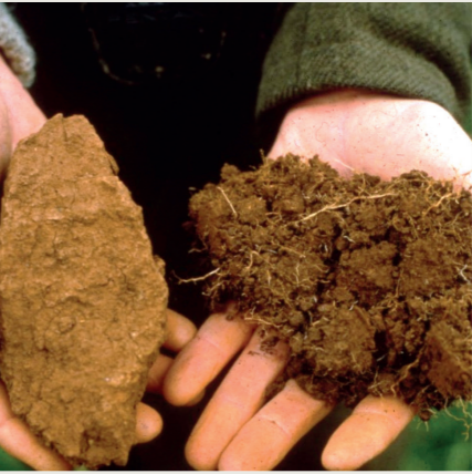
Figure 6. A handset soil horizon on the left compared to a well structured sample of the same soil on the right.
