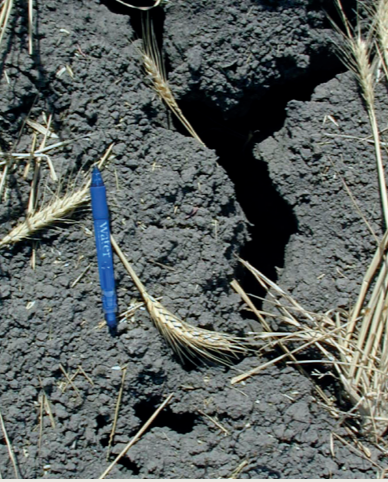
Figure 3. A uniform, grey clay showing the crumb surface structure and cracking typical of self-mulching soils.
