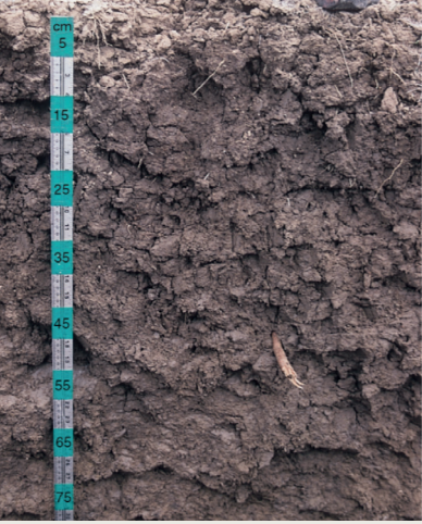
Figure 2. A uniform, grey clay showing the absence of any abrupt texture change within the profile.
