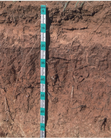
Figure 1. A texture contrast (duplex) soil showing a clay loam topsoil (0-25 cm) overlying a heavy clay subsoil.
