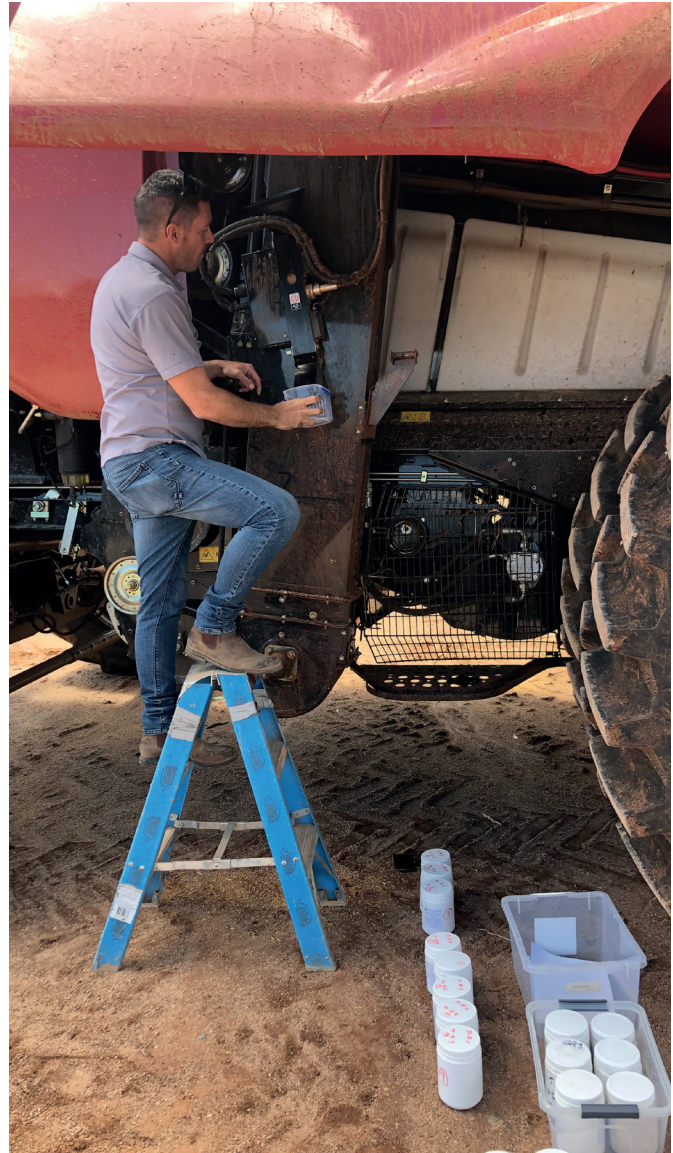
Figure 1: Mat Clancy (Next Instruments) performing a calibration on the CropScan 3000H unit at Ardlethan using reference standards of known protein percentage.
